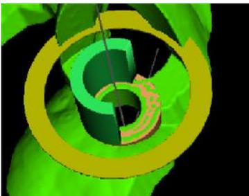
Click the Change Drill Stop Orientation. With the cursor near the drill stop in the 3D view, rotate the widget to reorient the drill stop.
